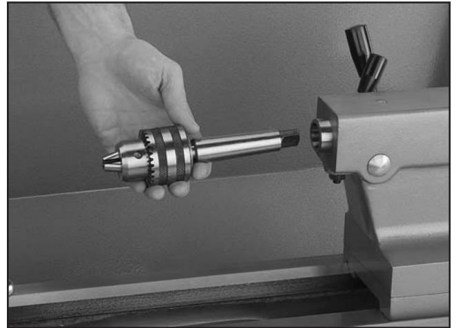
Figure 29. Setting up tailstock for drilling.
